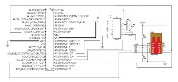
Figure (7) schematic circuit design of Master side
