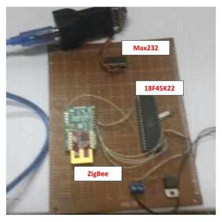
Figure (8) interface circuit design in Master Side
