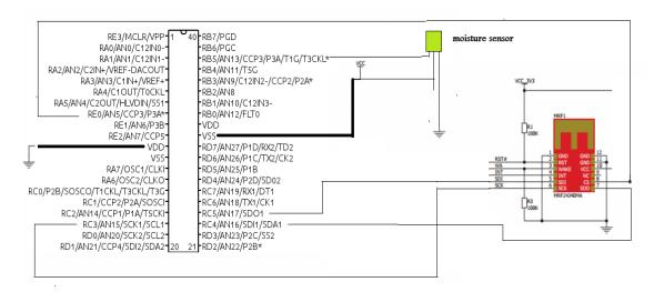
Figure (5) schematic circuit design of slave side
